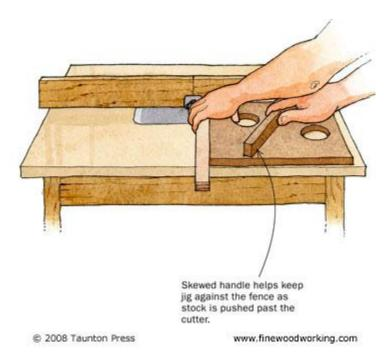
To use, simply hold the workpiece against the block and push through, keeping the block firmly against the fence. The block can be reversed to make a new zero-clearance backer, and it's easy to replace when it gets worn out.
