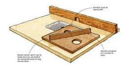
This router-table push block, or backer block as I like to call it, stabilizes the workpiece and reduces tearout. It is handy for backing up the cut across the grain, such as when profiling a panel, but it's especially useful for milling the ends of narrow stock, such as when cutting stub tenons in a frame.
